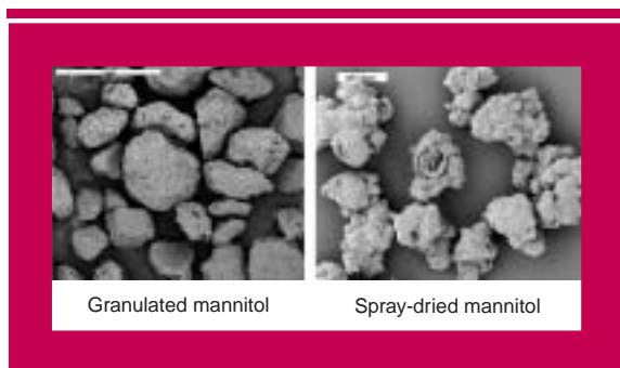
Figure 3: SEM micrographs of textured mannitols.
